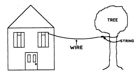
Tie the end of the antenna wire to a piece of string which in turn is tied to a tall object.
